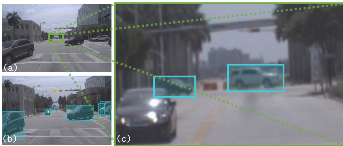
Figure 3.11: Detection of Far Away Objects: Our Two-Plane Prior boosts the detection of small far-away objects at lower resolutions (depicted image from Argoverse-HD dataset). The cropped green region in the (a) original image is (c) zoomed in while (b) shows all the detections in the warped image. Our method is able to detect the occluded car.
