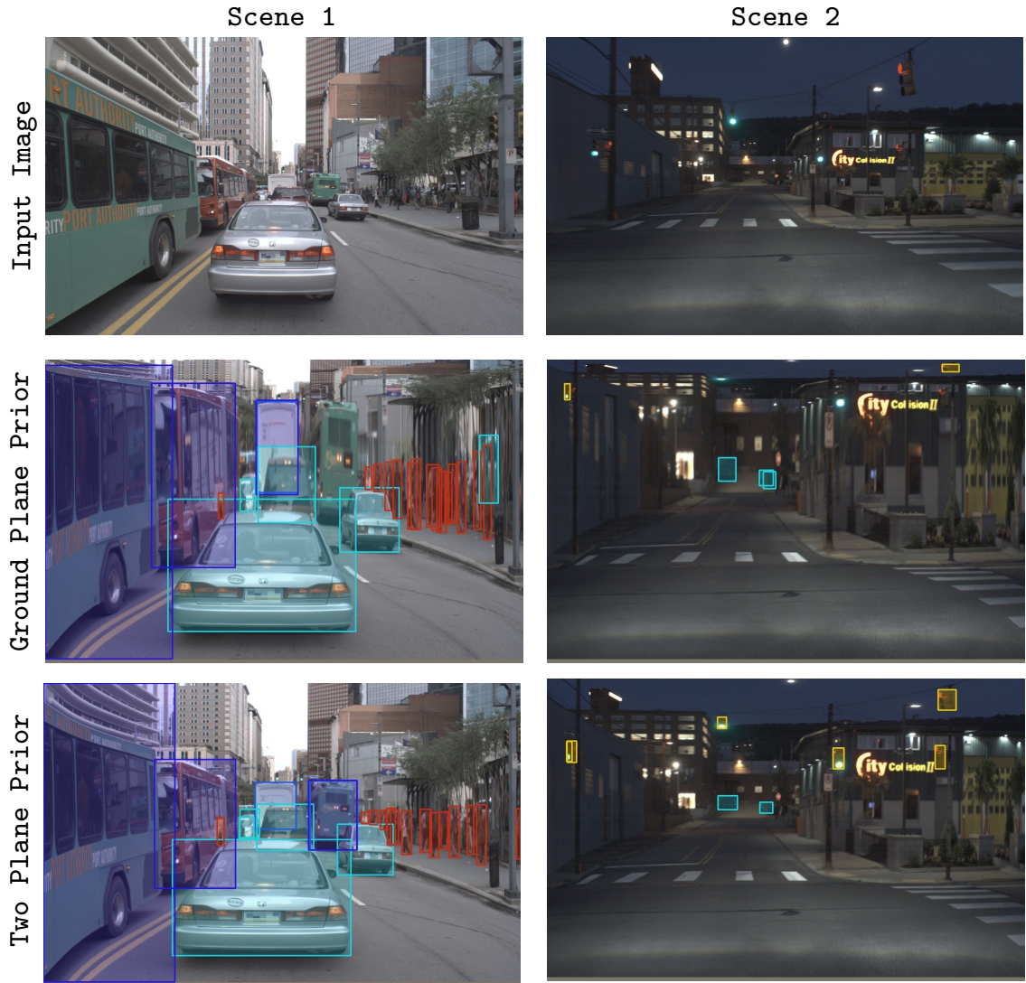
Figure 3.6: Ground Plane Prior vs Two-Plane Prior: This figure demonstrates how crucial it is to model the second plane. Learning is difficult with Ground Plane Prior (Section 5.1 in the manuscript) and causes heavy distortion of non-ground-plane regions.
