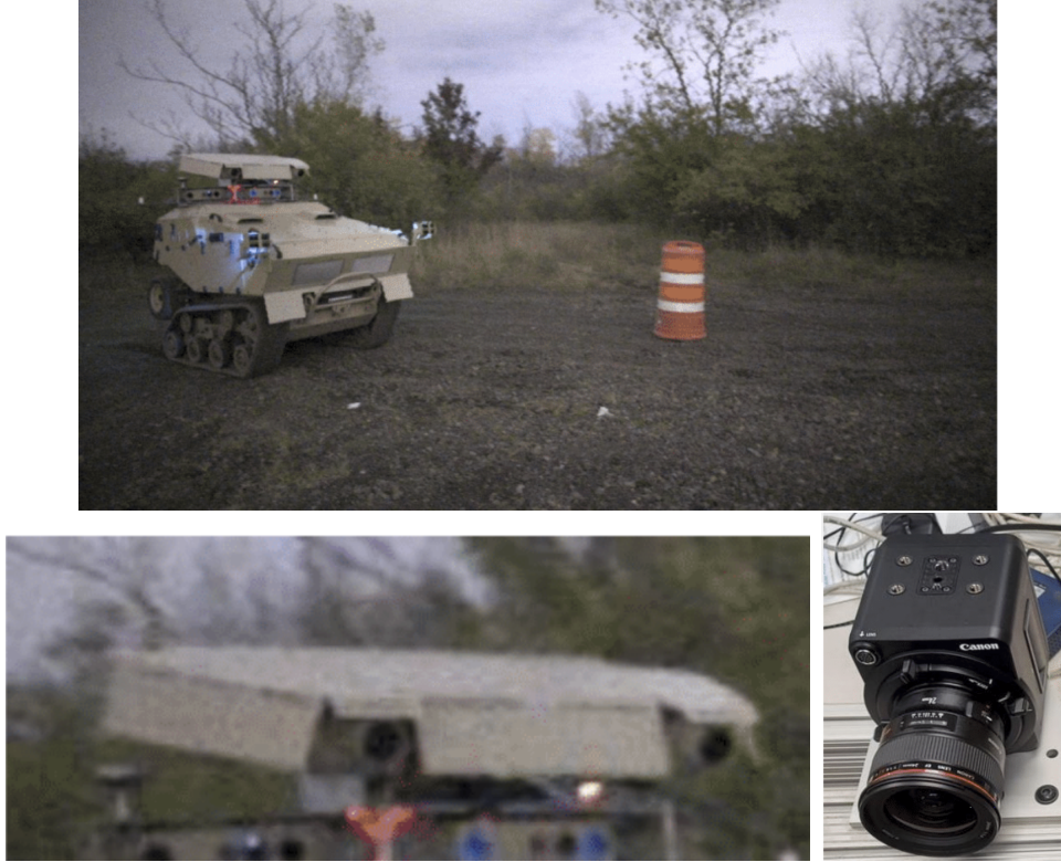
Figure 3.1: Our Robotic System with high-sensitivity cameras, Canon ME20F-SH (pictured bottom-right), for night operations mounted at the top.
