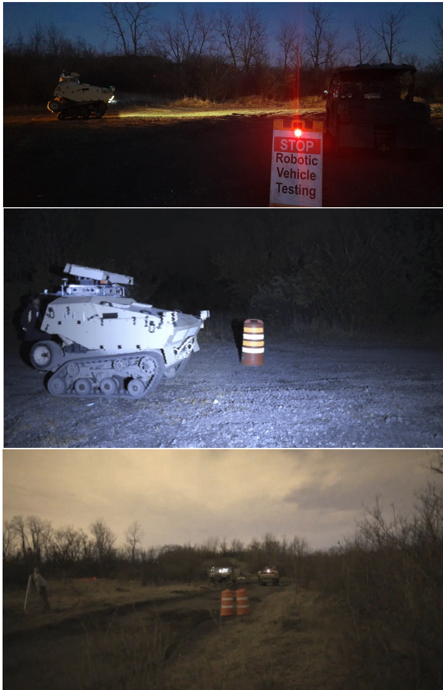
Figure 3.2: Images of our robot in our operating environment. The first corresponds to an image taken prior to start of operations, the second at time of operations illuminated with a flash-light to illustrate the surrounding darkness, and the third captured with another high-sensitivity camera during operation.
