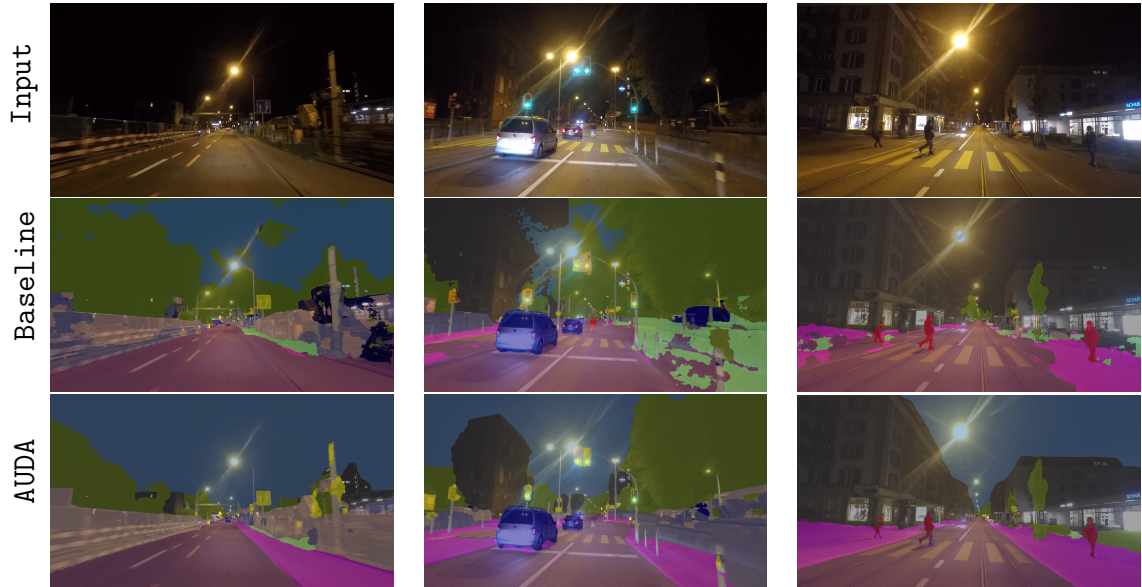
Figure 4.7: We can see significant improvement in these representative examples from CS \rightarrow DZ after AUDA. Our predictions are generally far smoother, performance particularly in background classes is far improved, and our model looks to be capable of operating in such night time environments.
