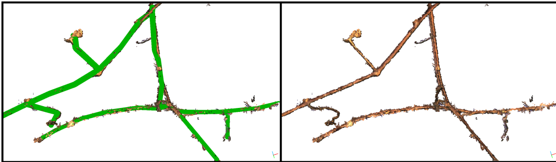
Figure 5.8: Lines are jointly optimized along the topological edges by minimizing point-to-line MSE between point cloud and skeleton as the line endpoints move. Left we have the estimated line segments with radii, right shows the underlying colored point cloud.
