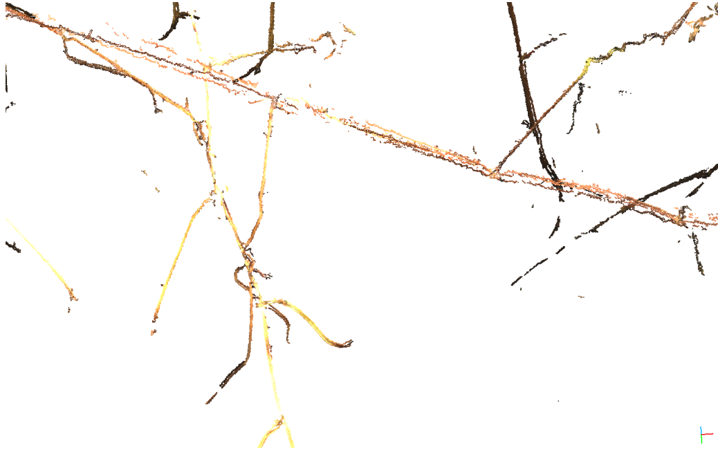
(c) Point cloud after dilation for precision improvements have been applied. As can be seen there are still some reconstruction issues, such as the separated cane portions running parallel, but a great deal of edge noise is eliminated.
