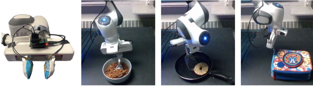
Figure 4.3: Tasks and hardware setup. We attach the Piezo contact microphones to our gripper (left), which record vibrations in the form of audio. We run experiments on three real-world tasks: scooping, spatula flipping, and zipping (right).
