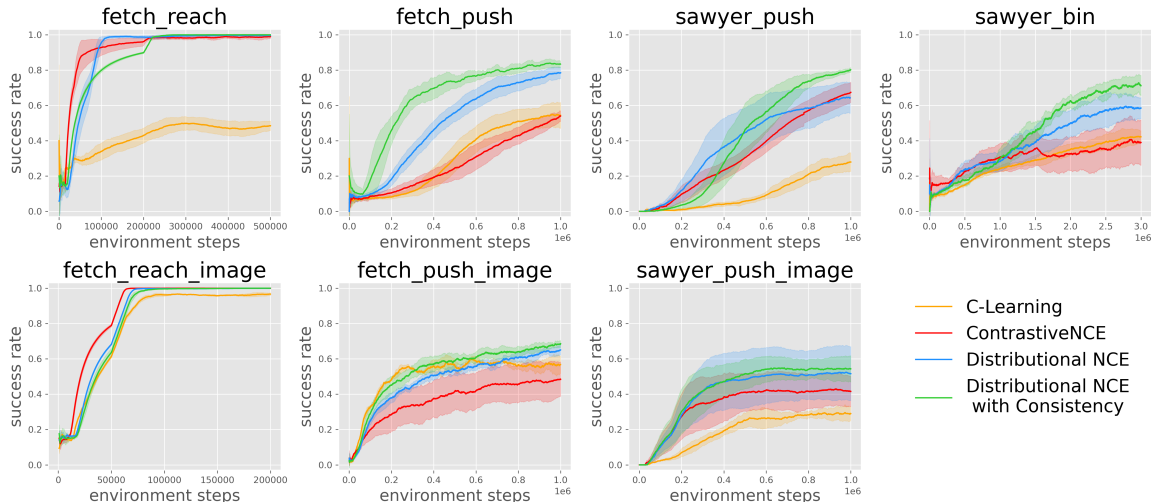
Figure 7.2: Comparison with baselines. Distributional NCE outperforms the Contrastive NCE [14] and C-Learning [13] in all but the easiest tasks ( fetch_reach , fetch_reach_image ). Applying temporal consistency on top of Distributional NCE accelerates learning and boosts asymptotic performance.
