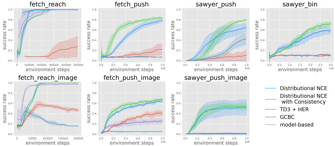
Figure 7.3: Comparison with (non-contrastive) RL baselines. Distributional NCE methods outperform the prior (non-contrastive) GCRL baselines, TD3+HER [2], Goal-conditioned behavior cloning (GCBC) [9] and model-based approach [8, 10, 24], across all the tasks.
