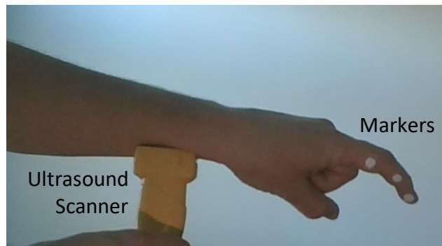
Figure 1. Setup for tracking the finger using markers via a camera, while scanning the muscles of the forearm with the Terason ultrasound scanner in an axial orientation.
