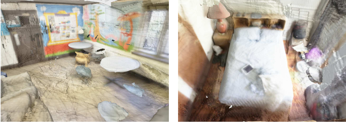
Figure 7.6: With scale calibration and volumetric fusion, room-scale geometry initialization can be achieved from monocular depth without any optimization of the voxel grid parameters. The remaining task would be refining noisy regions and prune outliers.
