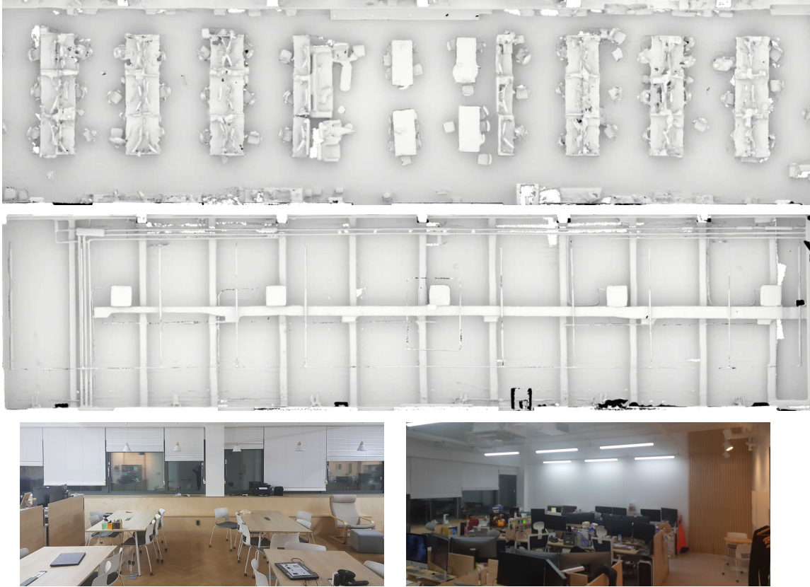
Figure 6.2: Surface reconstruction via SDF integration of the lab sequence from LiDAR range images. Top and bottom left are the ground and the ceiling rendered with Mitsuba 2 [172]. Bottom right are pictures of the scene.
