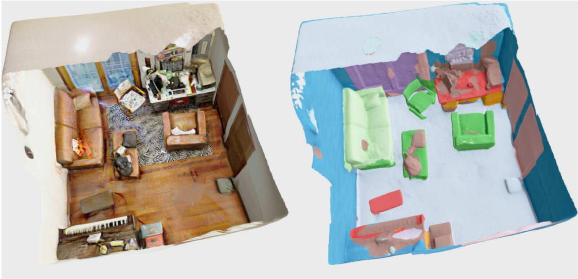
Figure 7.1: Color and semantic scene reconstruction from our system with monocular images and learned monocular priors.
