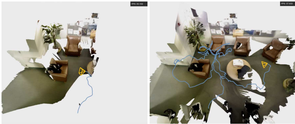
Figure 5.14: Visualization of the real-time dense SLAM system in the quality mode with colored and interactive surface reconstruction. Viewpoints can be changed by users to visualize the incremental reconstruction of the scene.
