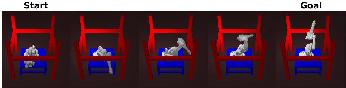
Figure 8.2: Kinodynamic motion planning for an ABB arm. Figure (left to right) shows waypoints along a plan.
