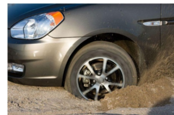
(c) failure due to soil shear is evident. Though the wheel may be spinning, the soil cannot provide the required normal force necessary to support the vehicle's forward movement [95].
