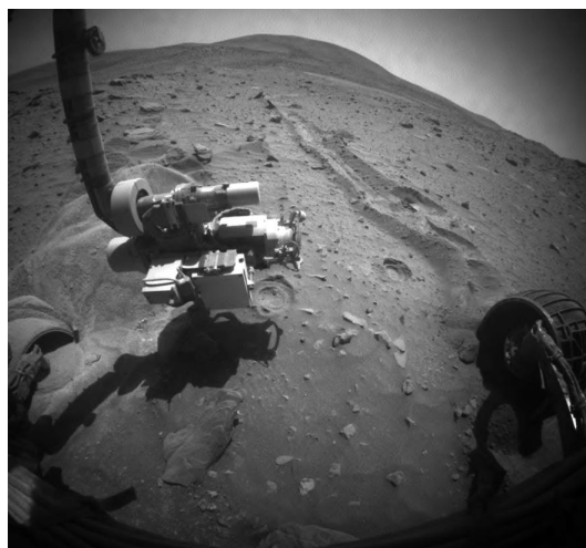
Figure 1.3: Mars rover Spirit immobilized in martian soil [11].
