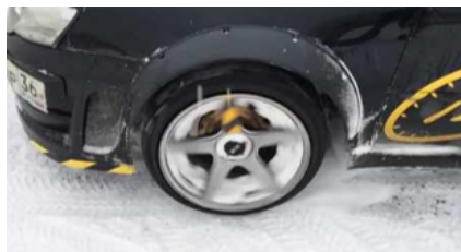
(b) This vehicle does not have enough traction to traverse the slippery ice due to the limited friction between the tire and ice [94].
