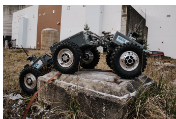
(a) A six-wheeled vehicle with articulated chassis designed by the Robotika team [2].
