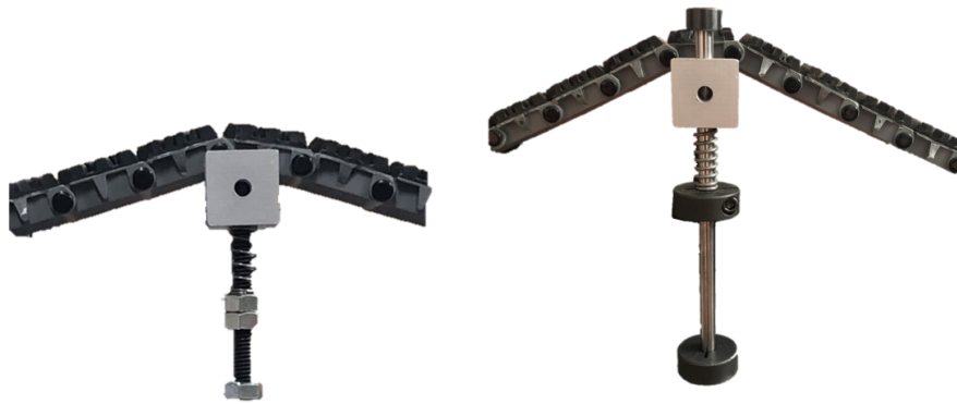
Figure A.8: Close-up view of old tension system (left) with bolts and nuts and new tension system (right) with shafts and shaft collars.
