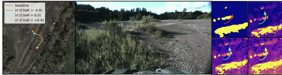
(a) Costmaps learned via IRL allow the robot to cut a corner over some low grass (about 15cm), while the baseline takes a longer route (note that obstacle inflation makes the grass patch appear as an obstacle to the baseline).
