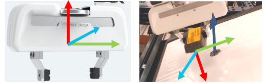
Fig. 2: Left: Palm keypoint with an arbitrary frame. Right: Tool keypoint with EE frame and surface normal (black arrow) for black mark on the board. The other in-plane axes for the black mark are much more arbitrary.
