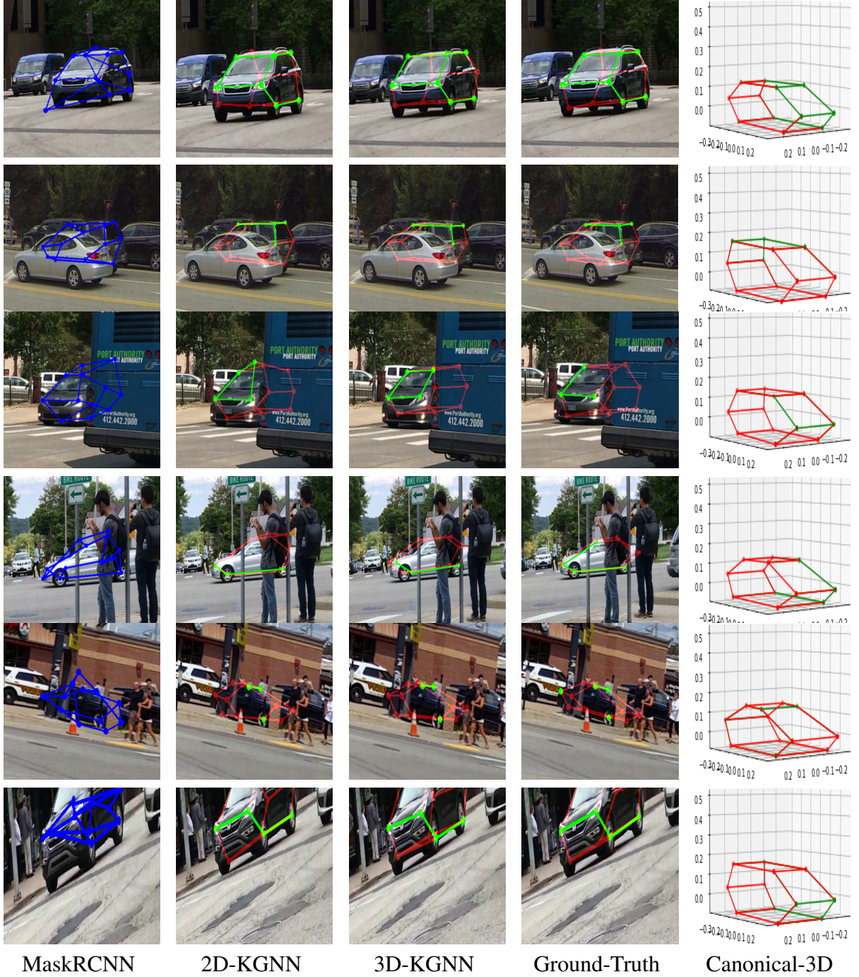
Figure 2.11: Qualitative evaluation of the 2D/3D keypoint localization for different occlusion categories of cars from the CarFusion dataset. The initial detector was trained using the MaskRCNN on the visible 2D keypoints. We use our self-supervised 2D-KGNN and 3D-GNN to localize keypoints from a single view. 2D reprojections of the 3D keypoints are shown in third column. The second and third columns show clear improvement in the localization of the occluded keypoints with respect to the baseline MaskRCNN. The canonical 3D views computed using 3D-KGNN are shown in the last column. The ground truth is obtained by applying trifocal tensor on the human labeled visible points to estimate the invisible points. Green represents visible edges and red represents occluded edges.
