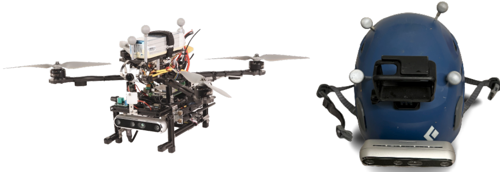
Figure 3.6: (Left) Aerial robot and (Right) helmet for the human partner used in the hardware experiments.
