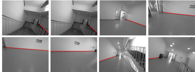
Fig. 1. An example of long-term line association. As lines are unbounded, they can generate long-term associations. This increases the correlation among poses, which benefits reducing drift, but may also significantly increase the runtime of the optimization if all the poses where a long 3D line segment is observed are jointly optimized. Thus it is important to design a scheme to balance the efficiency and accuracy. In addition, the line matching is also challenging. Since different parts of a line may be captured at different time, as demonstrated above, the feature-based matching scheme which is well-established for points is not suitable for lines.
