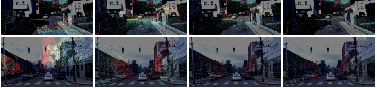
Fig. 4: Visualizations of the projected depth maps from KITTI Odometry dataset (upper row) and Argoverse Tracking dataset (lower row) (further distance is represented by red, closer distance is represented by blue) From left to right are initial pose, baseline with 0.1m voxel size, baseline with 0.2m voxel size and our HyperMap result. Best viewed in PDF file.
