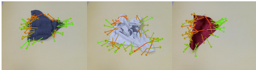
Supplementary Figure A.8: Examples of 50 sampled actions used for planning. Each arrow goes from the 2D projection of the pick location to that of the place location. The actions with the higher predicted reward are shown in greener color and the actions with the lower predicted reward are shown in redder colors.
