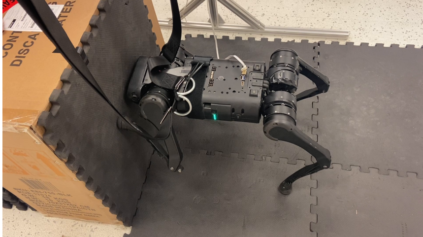
Figure 3.10: Hardware demonstration of the wall-leaning reference trajectory.
