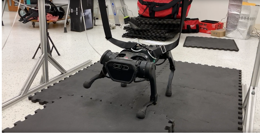
Figure 3.8: Hardware demonstration of the quadruped tracking of the box climbing trajectory.
