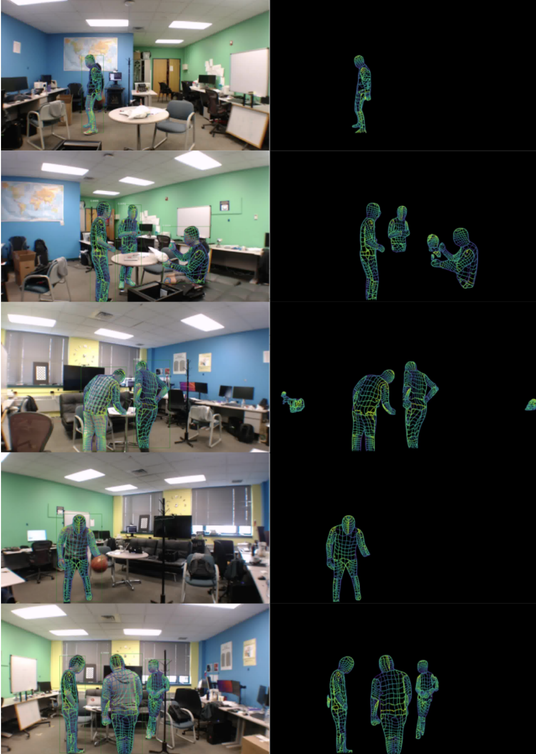
Figure 4.3: Qualitative comparison using synchronized images and WiFi signals. (Left Column) image-based DensePose (Right Column) our WiFi-based DensePose.
