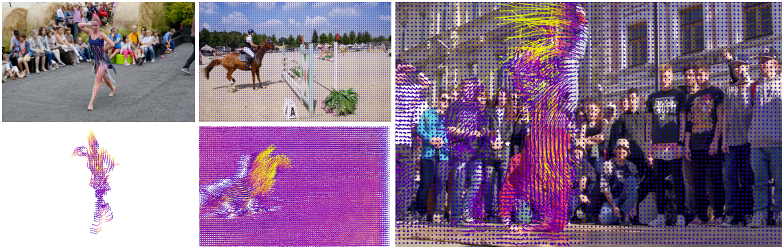
Figure 3.1: Persistent Independent Particles. Our method takes an RGB video as input, and estimates trajectories for any number of target pixels. Top-left: target pixels are marked with dots; bottom-left: estimated trajectories. Right: estimated trajectories overlaid on the first frame of the input video.
