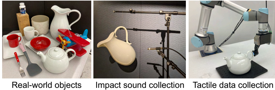
Figure 4.5: Illustration of real-world objects used in experiments and our hardware set-up for collecting real-world impact sounds and tactile data.
