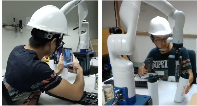
Figure 5.8: The robot presents a box in the wrong orientation, forcing the human to reach far to scan the box's label as shown on the left. The robot also almost knocks over one of the obstacles, a white bottle.
