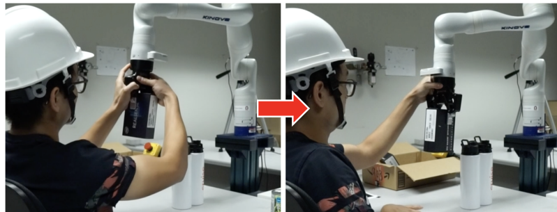
Figure 5.10: The human also perturbs the orientation of the box so that its barcode correctly faces the human.
