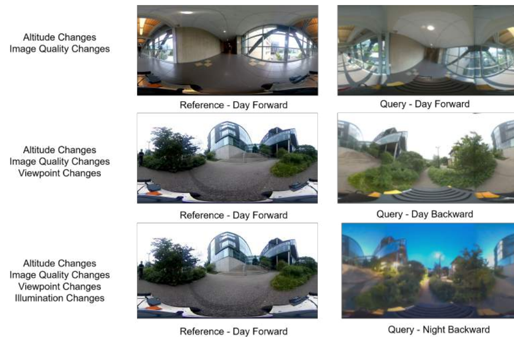
Figure 8.10: First row shows the the altitude and image quality changes between reference image from mapping robot and query image from the localization helmet. Second rows show adds viewpoint changes. Third row adds illumination changes.
