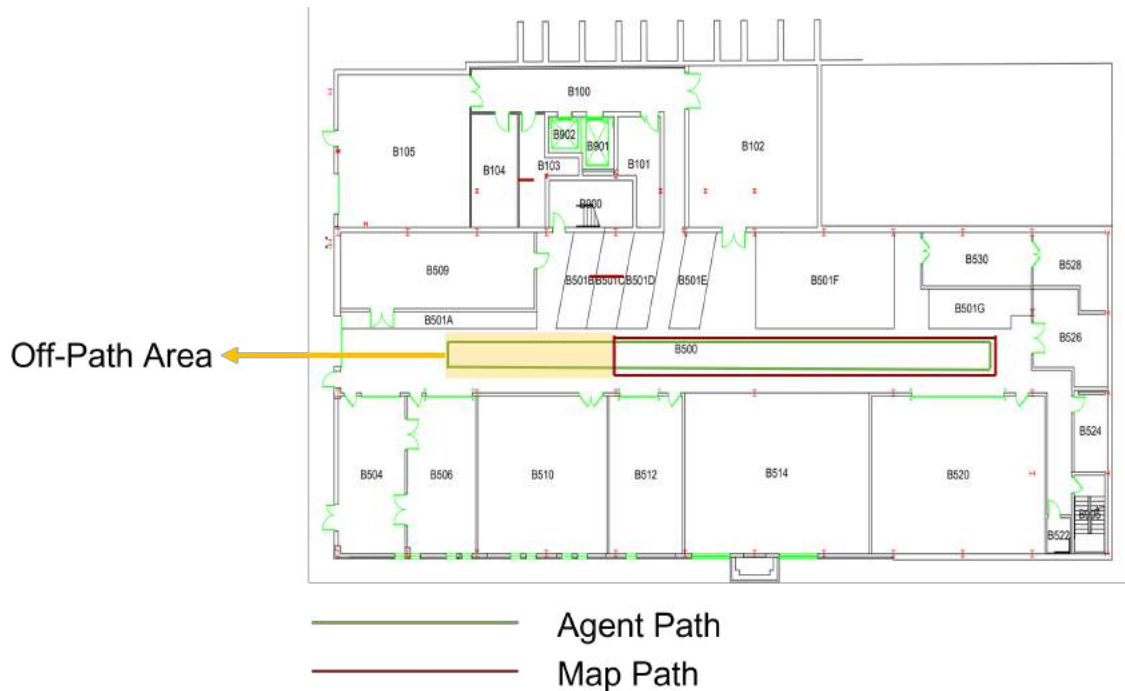
Figure 5.5: The figure is an example of an agent’s movement, including off-path. The red line is the pre-generated map, and the green line is the agent’s path. When the agent enters the yellow-shaded area, he/she is off the map. When the agent moves out of the yellow-shaded area, he/she is back on the map again.
