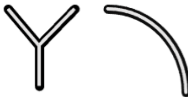
Figure 6.5: Contour types extracted from a skeletonized image. The black area around the gray skeleton is the contour.
