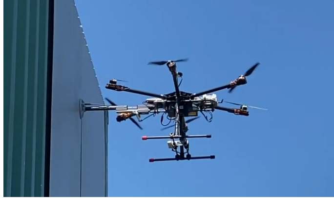
Figure 3.20: A fully-actuated hexarotor using the PX4 controller extended with our proposed design making an unmodeled contact with the wall.
