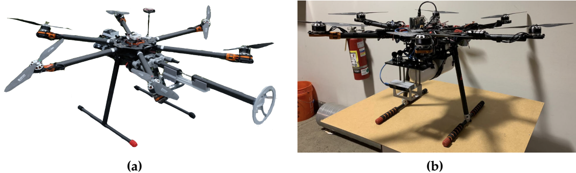
Figure 3.18: The fixed-pitch hexarotors used in our experiments. (a) The larger design with Tarot T960 frame. (b) The smaller design with Tarot X6 frame.
