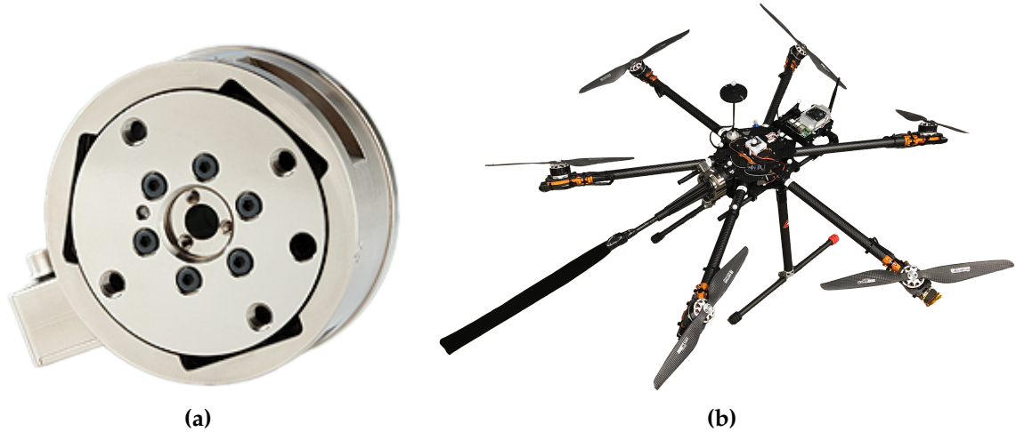
Figure 3.19: (a) Illustration of the ATI Gamma Force/Torque Sensor used for the force control tests [7]. (b) Our fully-actuated multirotor with the force/torque sensor attached.
