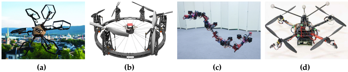
Figure 2.3: Some examples of variable-pitch fully-actuated multirotor designs in the literature. (a) [77] (b) [159] (c) [211] (d) [158].
