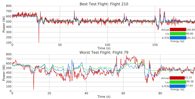
Fig. 4. Test Flights with the best and worst MAPE for b-TCN. The bar graphs in the bottom right corners represent the total energy estimate over the entire flight.
