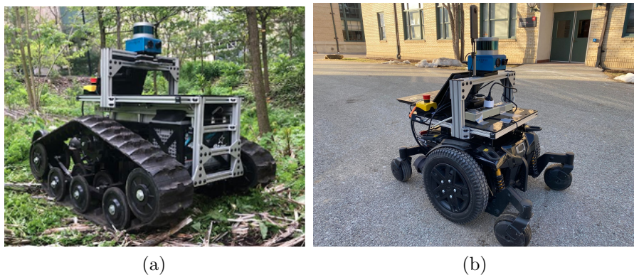
Figure 5.1: (a) The tracked vehicle used for data collection. (b) The robotic wheelchair platform used in the experiments equipped with a 4.1GHz i7 computer and a NVIDIA GTX 1660Ti GPU card. Both platforms are equipped with a Velodyne Puck Lidar, a MEMS-based IMU, and a monocular camera.
