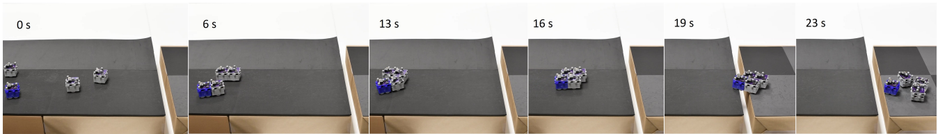
Fig. 6: Screenshots of four robots coupling to form a mesh configuration, crossing the gap, and decouple.
