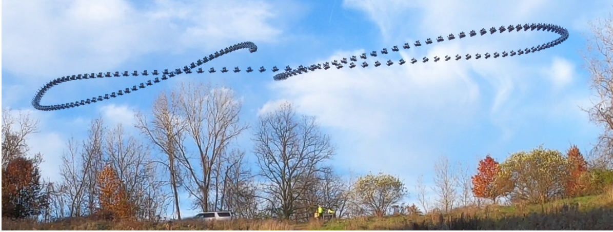
Figure 1.2: An example high speed trajectory executed outdoors on a quadrotor using our proposed methods.
