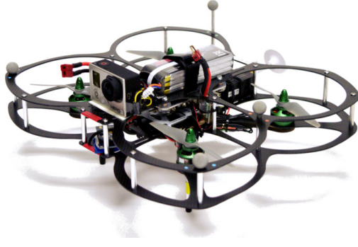
Figure 3.5: The 750g quadrotor used for the hardware experiments. Onboard computation is performed by an Odroid XU4 and the Pixhawk 1 Flight Controller.
