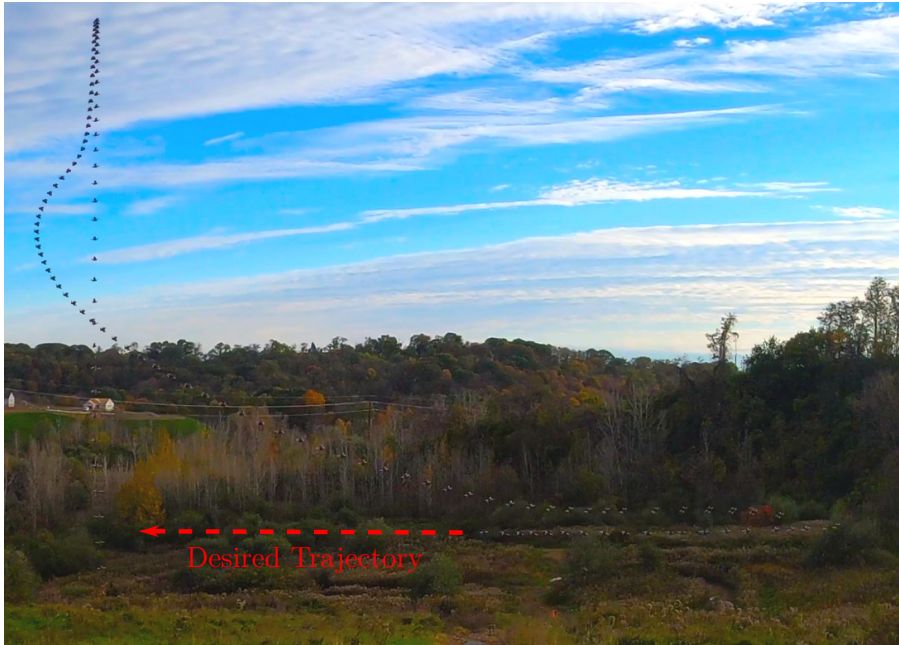
Figure 6.4: The vision-based estimates from the T265 experience extreme drift in the z -axis, which leads to a deviation from the desired trajectory and eventual crash.
