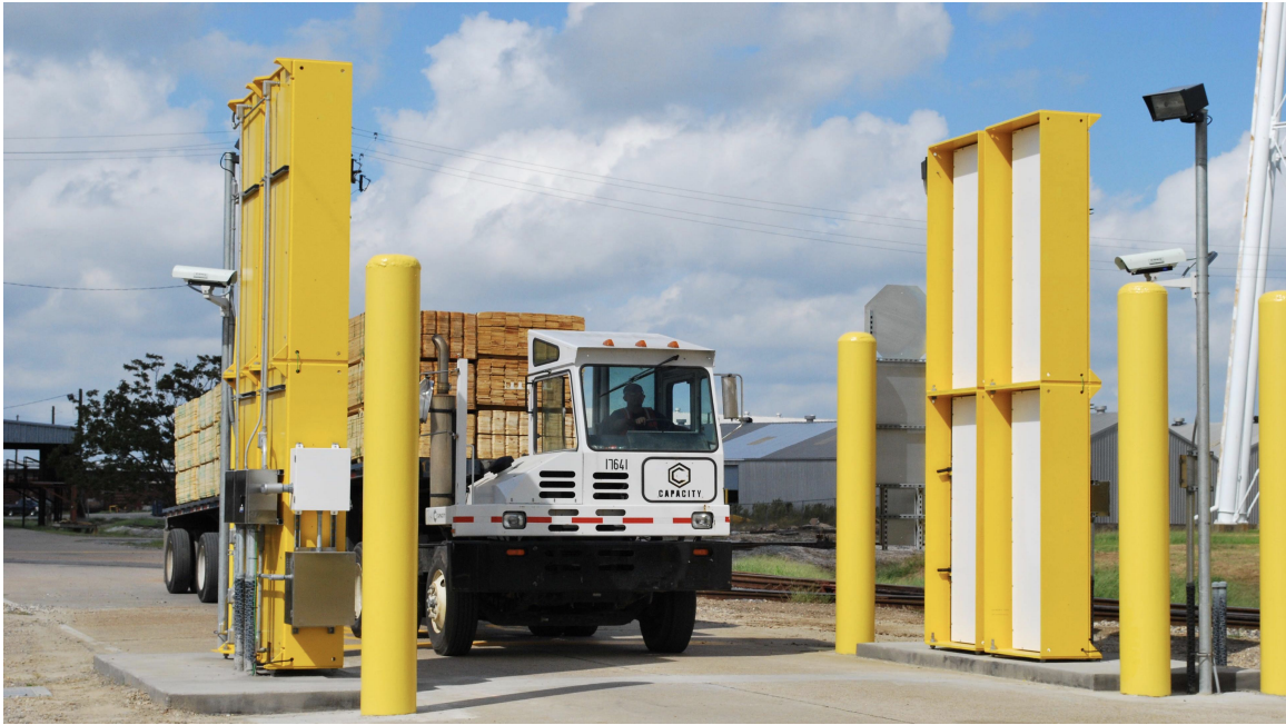
Figure 3.5: Radiation Portal Monitor in a Radiation Safety Context
