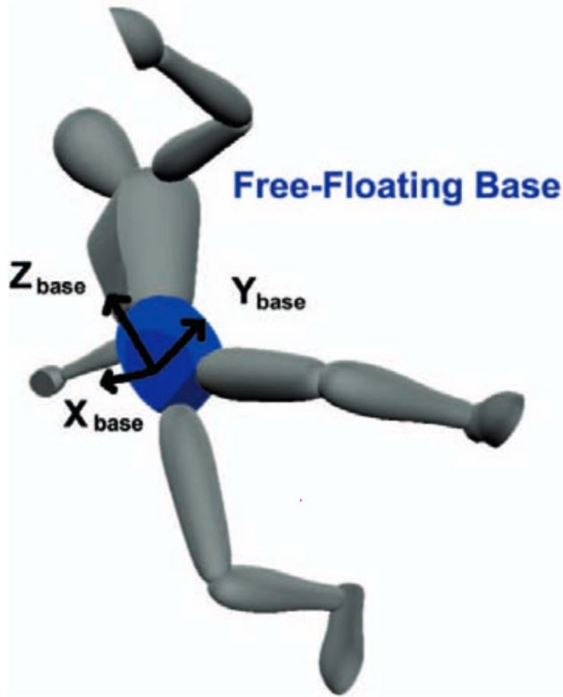
Figure 2.3: [22] developed an OSC formulation for floating base systems. Their test system was the above humanoid model. For their application, the operational space frame is the base frame located in the hip link of the humanoid robot. So for the humanoid OSC, joint torque commands in the legs and arms are computed to achieve a desired behavior in the base frame. For our space robot work, we define the operational space frame to be the end effector of the robot arm instead of the base link. Image from [22].
