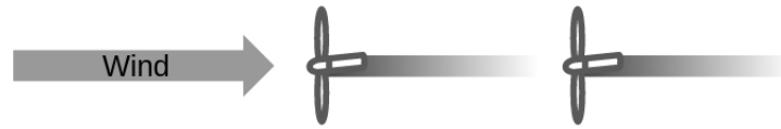
Figure 1.2: Two turbines in serial configuration relative to the wind, or aligned in a column, with wakes shown
