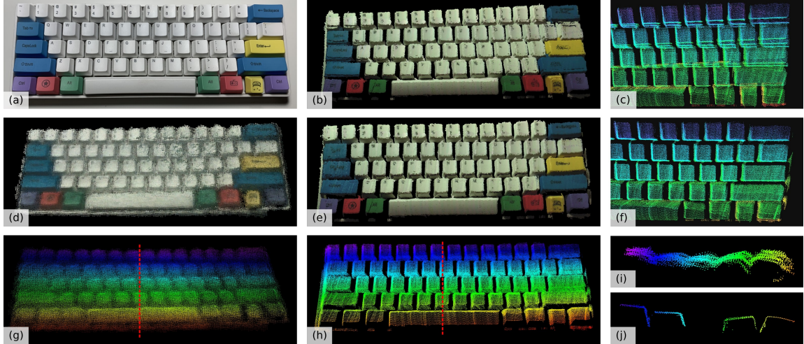
Figure 6.3: Comparison of point cloud reconstruction. (a) is a photograph of the scanned scene. (d) and (g) are the photo-realistically and spatially colored reconstruction results by RealSense. Reconstructed using the proposed sensor, (b) and (c) show results using VLI-Odom, and (e), (f) and (h) are with VLI-SLAM. (i) and (j) are the sectional views of (g) and (h) respectively with the red dashed lines as the cutting planes.
