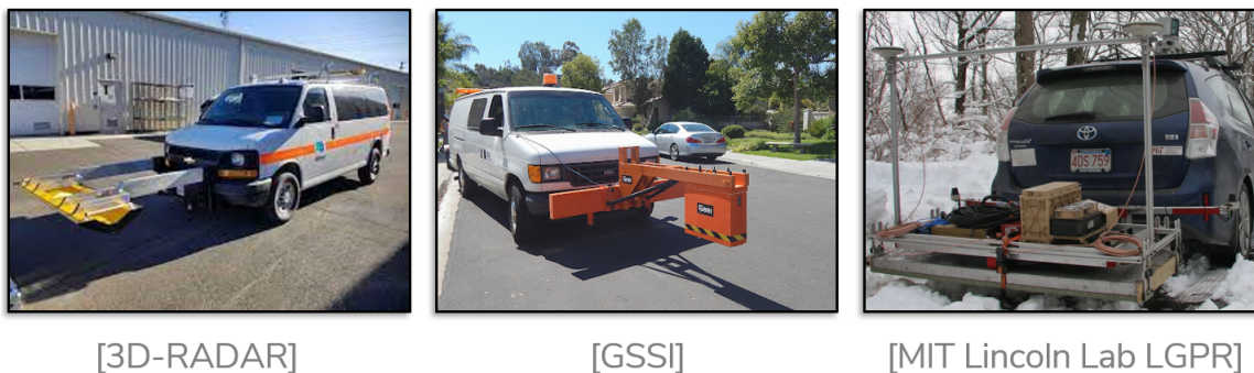
Figure 6.1: Different air-coupled and multi-channel GPR systems from [1, 2, 80] respectively.
