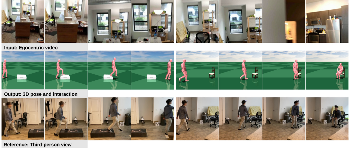
Figure 1.1: From egocentric videos, we infer physically-plausible 3D human pose and human-object interaction.
