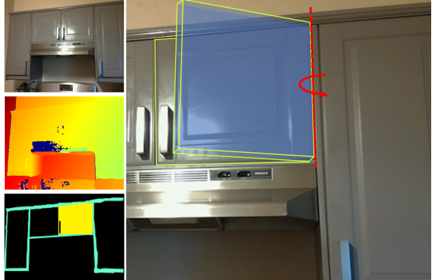
Fig. 1: Predicting articulation mechanisms using FormNet. Given the inputs on the left (RGB-D image and segmentation masks of a pair of object parts), a neural network predicts the articulation type (revolute, prismatic, fixed, or unconnected) and appropriate articulation parameters (e.g., location and direction of revolute axis). The network is trained on synthetic data and infers articulation parameters via predicting motion residual flows.
