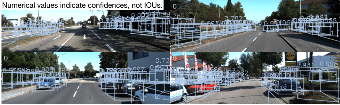
Figure 4.4: Ablation of ensemble agreement causes divergence. The model eventually detects objects everywhere.
