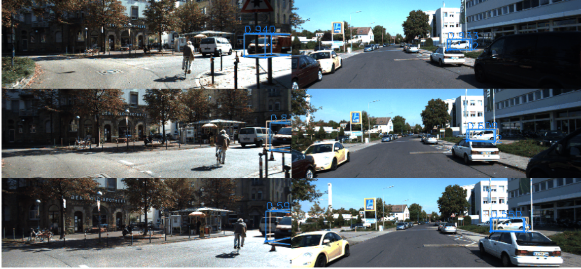
Figure 4.3: 3D object tracking in KITTI . IoU scores are marked alongside each estimated box (in blue) across subsampled frames.
