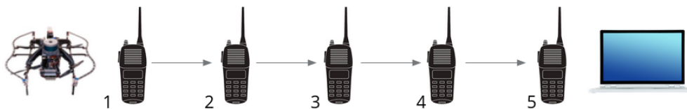
Figure 4.1: Example communication node topology with 5 nodes in a linear chain
