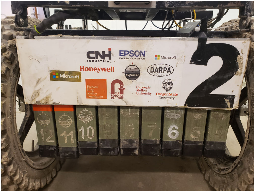
Figure 1.3: Node dropper loaded with 9 node casings each holding a Rajant DX2-50 radio
