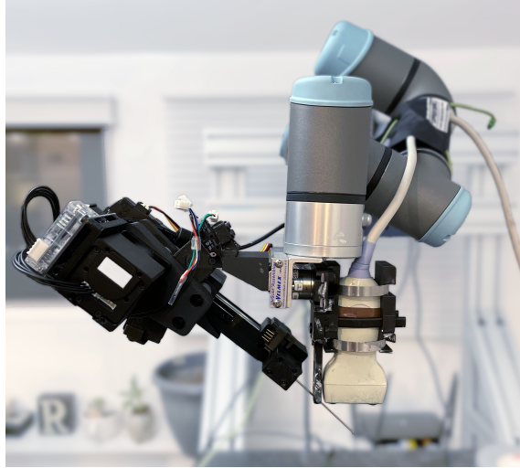
Figure 4.1: The two degrees of freedom (DOFs) needle insertion mechanism mounted to a UR3e arm along side an ultrasound probe.
