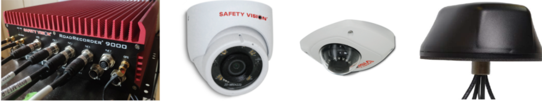
Figure 3.7: Pictures of the Hardware. (From left to right: bus computer; exterior camera; interior camera; GPS and network antenna.)
