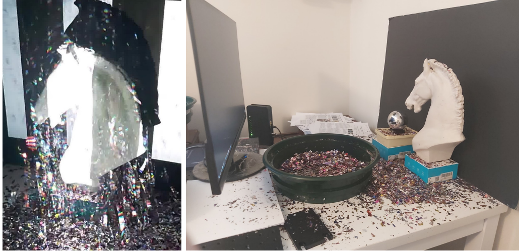
Figure 3.34: Left: Image frame showing the effect of confetti while scanning with our setup. Right: Setup image taken after scanning the object in the presence of specular noise-generating confetti particles.
