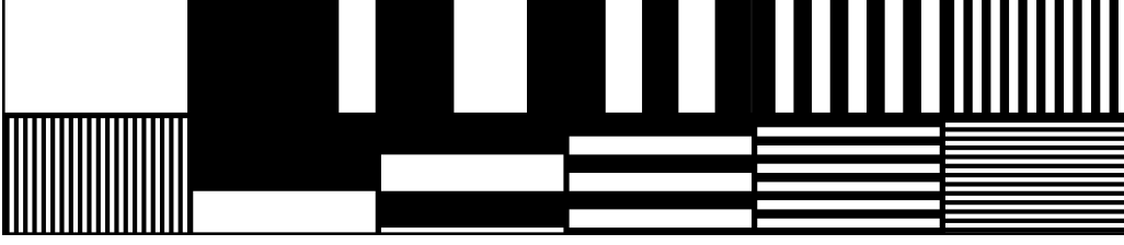
Figure 3.5: Generated binary gray code patterns used for structured light scanning.
