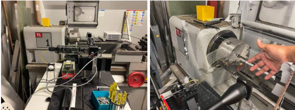
Figure 4.17: Left: Our shape from silhouette ballistic scanning setup on a Haas TL-1 CNC lathe. Right: Transparent acrylic sheets used to prevent our setup from fluids.
