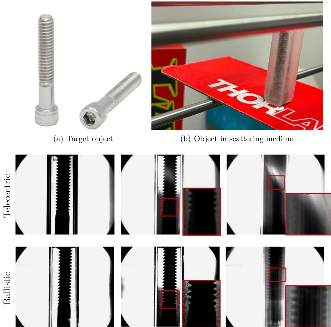
Figure 4.11: Silhouette capture results for a screw using telecentric and our ballistic scanning method in different concentrations.
