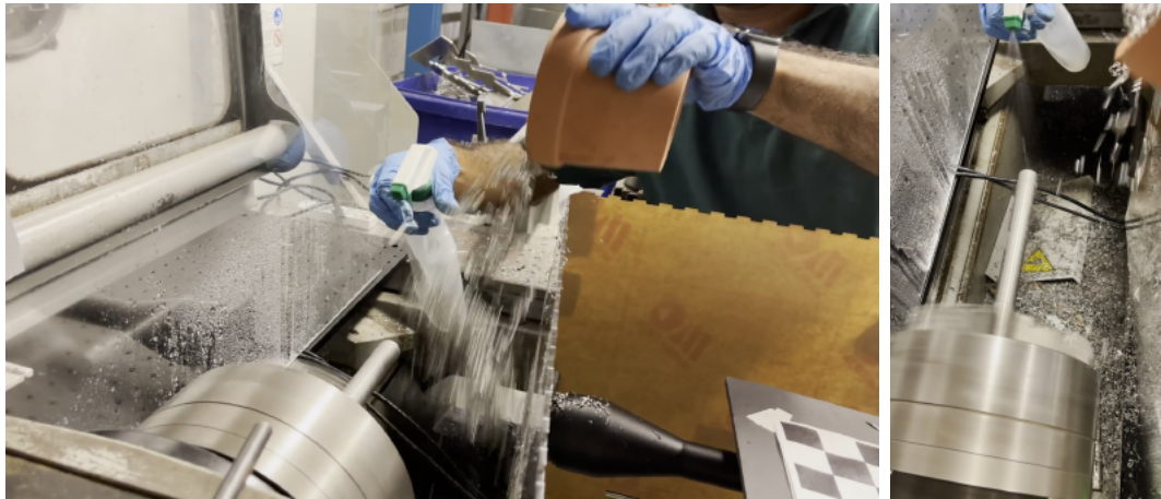
Figure 4.23: Fluid and specular chips being introduced in our scanning environment.
