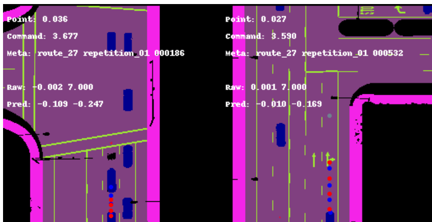
Figure 3.2: BEV images ( M_t ) of two samples. Agent is at the center-bottom of each image facing upwards. Red dots are LBC predictions f_{\theta}(M_t) , blue dots are ground truth w_t .
