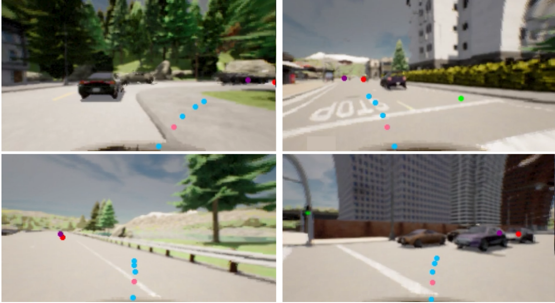
Figure 3.9: Top and bottom right: agent makes intersection turn too narrow and wide. Top left: agent chases the route waypoint off-road. Bottom left: agent mistakes highway shoulder for lane
