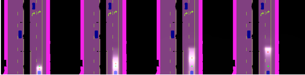
Figure 3.3: Visualizing each of the T heatmaps in b_\theta(M_t) which has output shape (T, H, W) . Each (H, W) heatmap is plotted in white over M_t .
