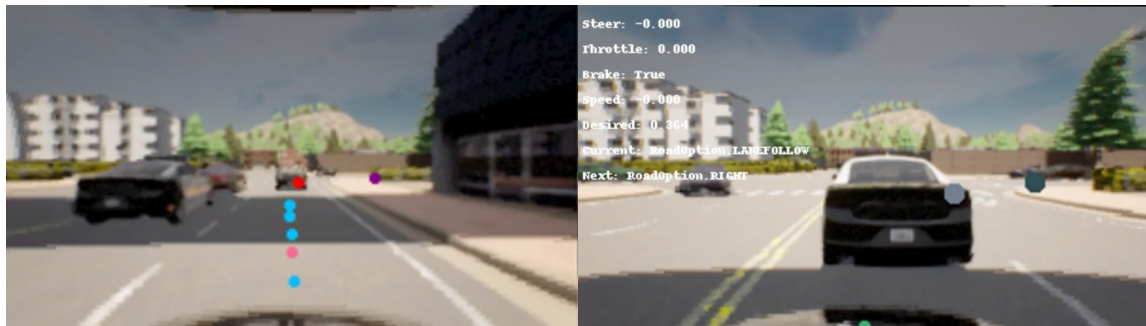
Figure 3.12: Left: baseline is in the correct lane. Right: margin agent is in the wrong lane, but is able to avoid stop infraction
