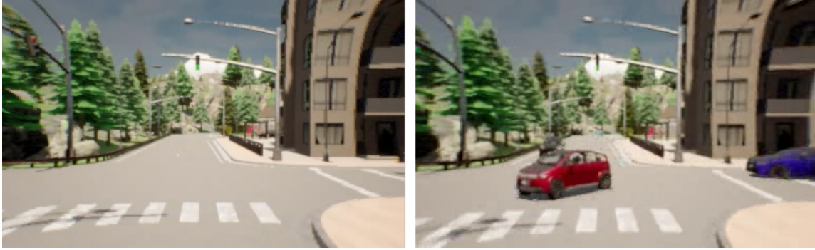
Figure 4.6: Left: blocked agent does not trigger scenario. Right: blocked agent that inched slightly forward triggers cross-traffic
