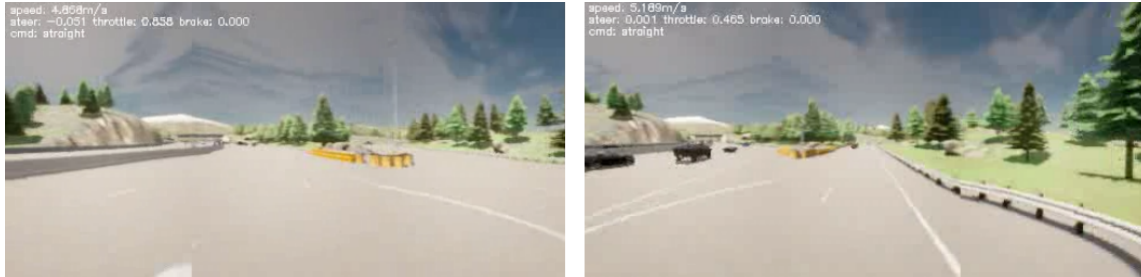
Figure 5.1: Right: agent A erroneously takes the highway exit, leading to route deviation termination. Left: agent B avoids the exit by being in the wrong lane.
