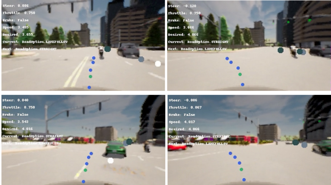
Figure 3.17: Top: In left image, agent drifts left and deviates from going straight in the right image. Bottom: Similar sequence of events that occur on a different intersection
