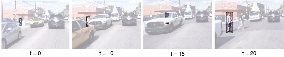
Figure 1.1: We visualize an online tracking scenario from Argoverse [10] that requires tracking a pedestrian through a complete occlusion. Such applications cannot wait for objects to re-appear (, as re-identification approaches do): autonomous agents must properly react during the occlusion. We treat online detection of occluded people as a short-term forecasting challenge.
