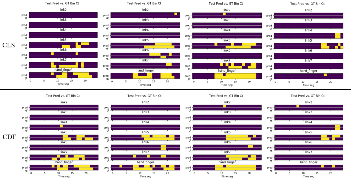
Fig. 9: Contact Detection Visualizations on Test Data. Each column is the execution of one trajectory. The top row have plots corresponding to predictions made by CLS, and the bottom CDF. In each plot, link-wise ground truth and predicted binary contact detections are visualized, with purple representing negative contacts, and yellow positive contacts. The X-axis represents prediction time segments, so each unit corresponds to 5 observations, one made every 4 simulation steps. In general, CLS has more FNs, and CDF has more FPs, which is consistent with results in Table I.
