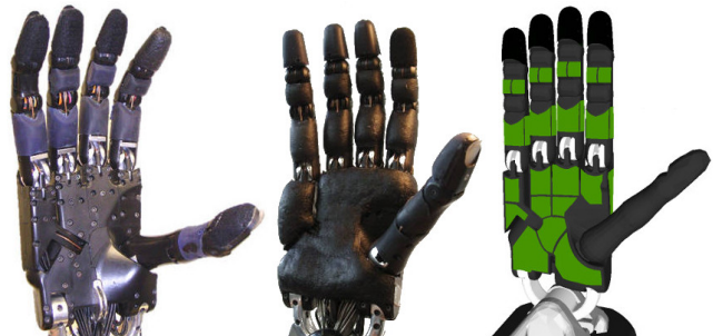
Fig. 2. A Shadow Dexterous Hand (left) that has been covered with a tactile skin [51] (middle) in order to provide tactile information at several locations (highlighted green regions on the right rendering).
