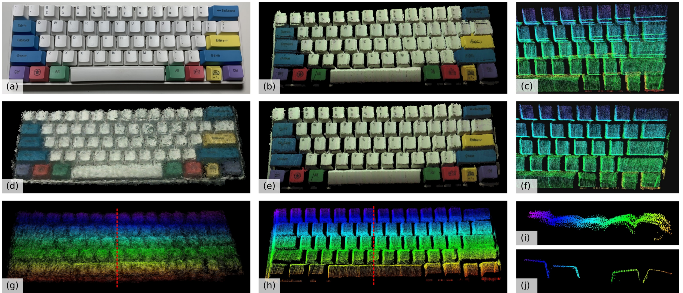
Fig. 7. Comparison of point cloud reconstruction. (a) is a photograph of the scanned scene. (d) and (g) are the photo-realistically and spatially colored reconstruction results by RealSense. Reconstructed using the proposed sensor, (b) and (c) show results using VLI-Odom, and (e), (f) and (h) are with VLI-SLAM. (i) and (j) are the sectional views of (g) and (h) respectively with the red dashed lines as the cutting planes.
