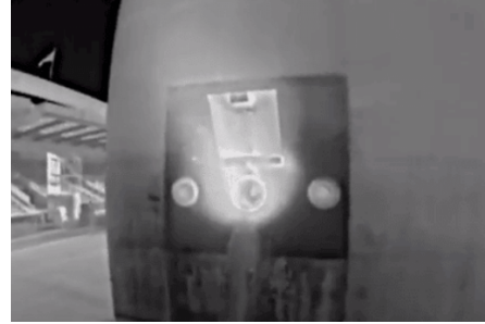
(a) Thermal image during competition, with sprayed water towards the fire but hitting below the opening
