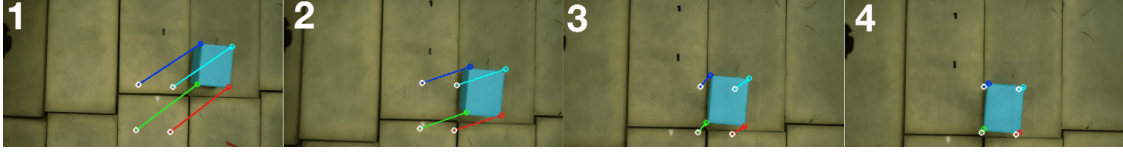
(a) Visual servoing over a block during a test in Pittsburgh, PA. Colored circles and lines represent the detected corners and pixel errors to the white circle goal coordinates.
