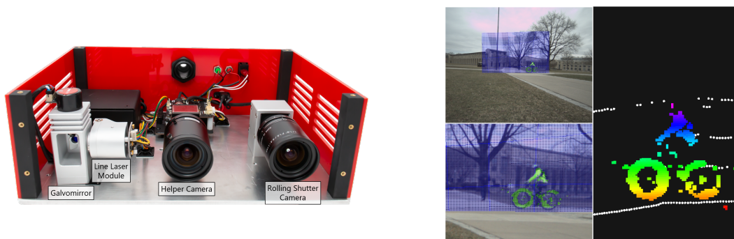
Figure 2.1: The Triangulation Light Curtain device, consisting of a steerable laser, an IR camera and a microcontroller, capable of generating a slice in space to image in 3D
