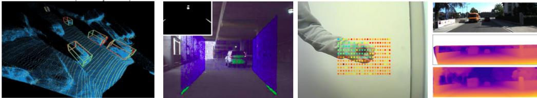
Figure 1.2: 1: Traditional LIDAR based depth and object detection [32] 2: Triangulation Light Curtain focusing its depth on the vehicle ahead [31] 3: MEMS based Lidar focusing its depth sensing pixels on the hand of the person [24] 4: RGB based depth estimation using the KITTI dataset
