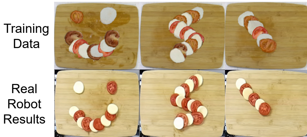
Figure 3.10: Our real world arrangement results when using our overall pipeline compared to the training images. The placement predictions for the real robot results shown used our local weighted PoE models described in 3.3.1.
