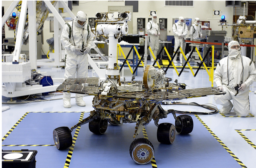
Figure 2.4: Spirit was the second rover to successfully reach Mars after Sojourner in 1997. It was also one of the first mobile robots to rely on visual odometry for localization.
