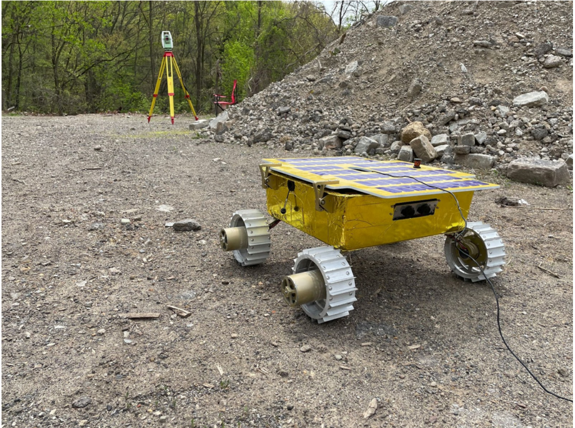
Figure 7.6: The surrogate rover being tracked by the surveying instrument in the outdoor test.
