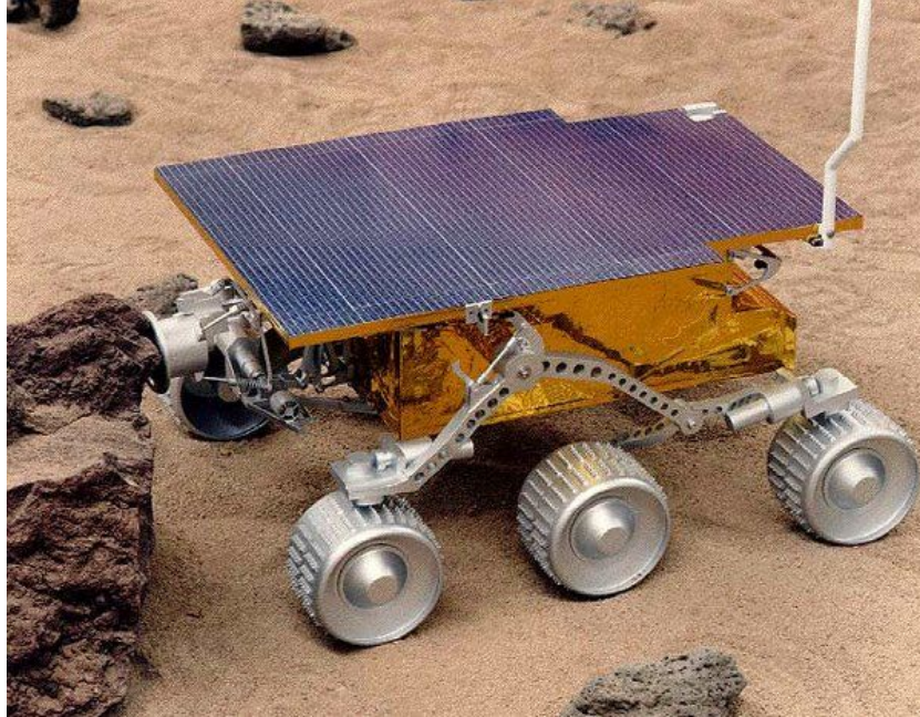
Figure 2.2: Sojourner was the first rover to roam another planet. Similar to modern space micro-rovers, the 11.5 kg rover was intended to operate only for a 7 day mission, drawing power from its solar panel and non-rechargeable battery.
