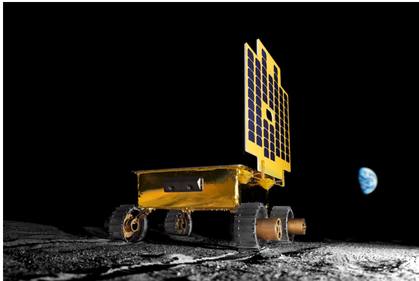
Figure 3.1: MoonRanger has a solar panel mounted on one side because of the low incident angle on the lunar poles.
