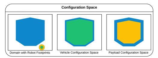
Figure 3.7: Choice of Vehicle and Payload Footprints Affects Configuration Space
