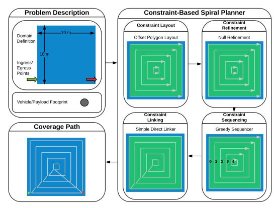
Figure 3.12: Sample implementation of spiral coverage within CB-CPP framework
